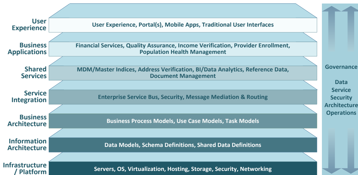
Figure 1 Layer View of HHS 2020 Technology Architecture
